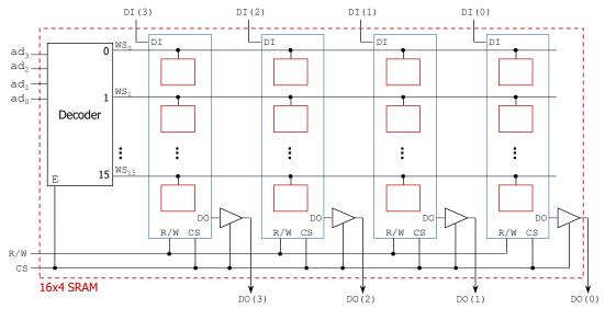
3-state output buffers: They are included to optimize implementation of larger SRAMs. If we want to build a larger SRAM out of smaller SRAMs (see memory decoding), we then do not need to use a large multiplexor:
