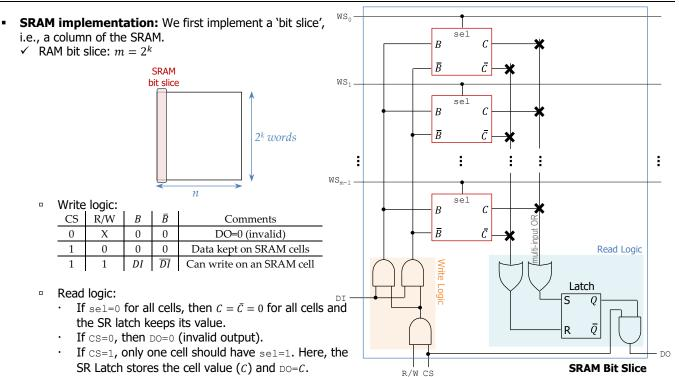
✓  $2^k \times n$  words SRAM: It can be implemented with a group of SRAM bit slices. For example: 16x4 SRAM (*n*=4, *k*=4).
