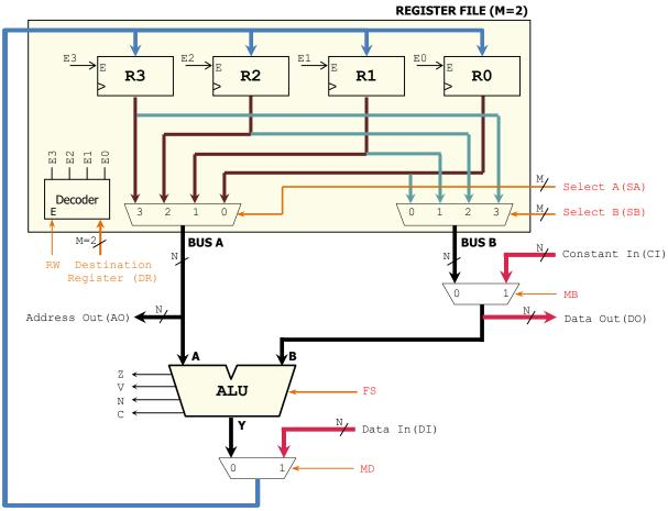
• Arithmetic Logic Unit: The FS has 4 bits, and the following table lists all the possible operations. The input Data (A, B) and output data (Y) are represented as signed numbers. Here, the flags Z, V, N, C are generated.
