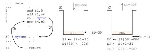
✓ <u>Example</u>: Nested subroutine calls (2 levels): Program Flow and Stack state. Note how the Stack structure allows to save (and restore) the PC values in the right order.
